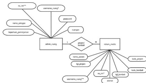
Gambar 10. ERD ( Entity Relationship Diagram ) hubungan III admin ruang.
